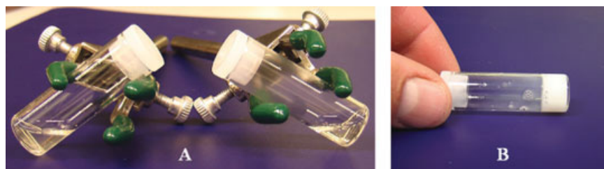
Figure 4 Photographs of (A) PVA-HY and PVA-AL solutions in water before mixing and (B) 1 min after their mixing. Both solutions contain 5 wt % of the PVA component. [Color figure can be viewed in the online issue, which is available at www.interscience.wiley.com .]
